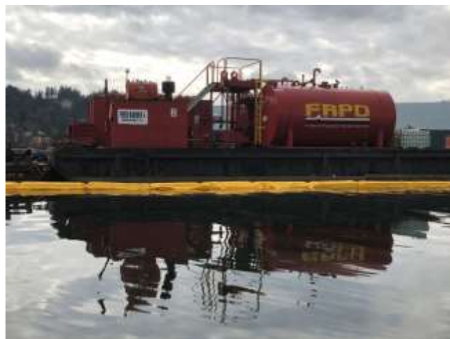
Bulk fuel storage barge. No sheen (spill) observed on water surface. Note: silt curtain (yellow) temporarily stored around barge.
