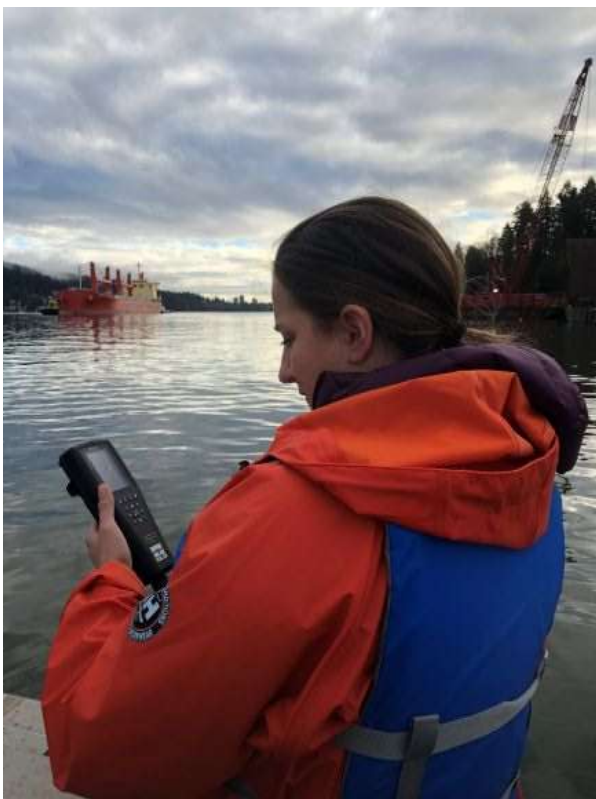
Daily open water turbidity monitoring using YSI handheld meter including probe on cable positioned to planned depths. Depth (surface, 1m, 3m and reference at 5m) readings are entered into mobile forms on an Ipad submitted on the internet to the Envirochem ENVOLV database for storage and reporting.
