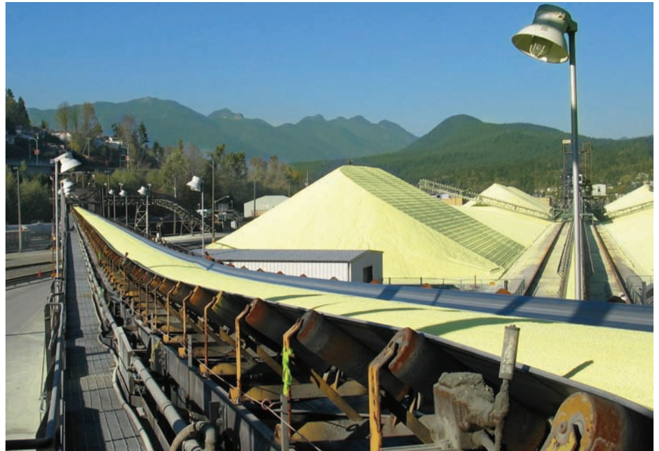
The Conveyor System Moves Sulphur From the Rotary Dumper to the Shiploader
