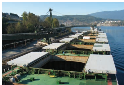
Bulk Carrier from above: the ships that come to PCT usually have seven giant hatches, or holds, in which the sulphur is loaded and transported.
