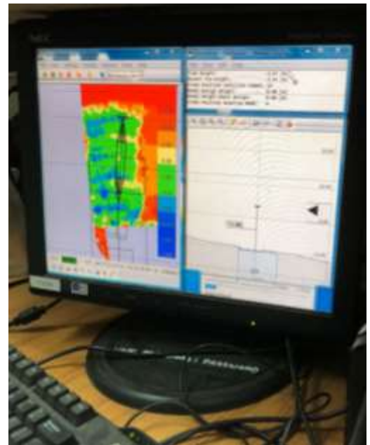
Qinsy software used by operations to control dredge cut (e.g., green-blue is target 0.5m depth on ground).
