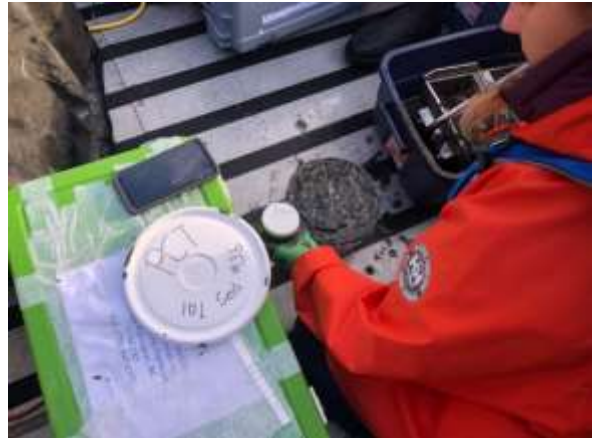
PAH affected sediment ponar sample to be submitted for DAS chemical analysis.
