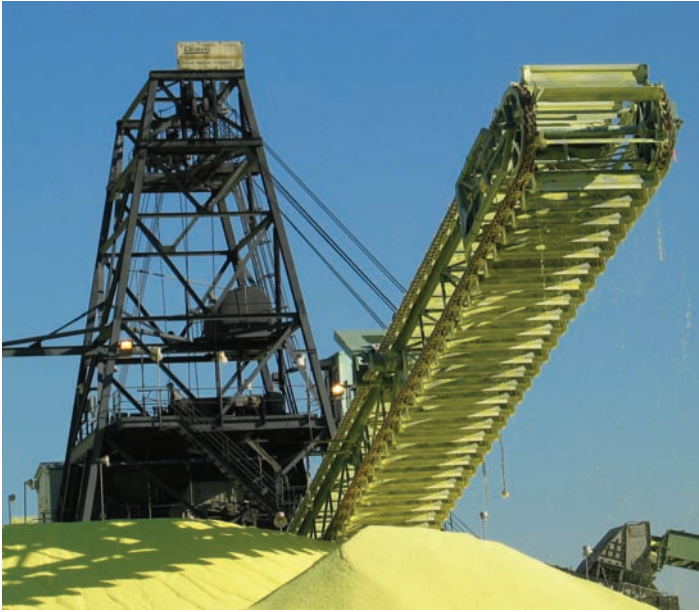
The booms on this stakrake will be replaced as part of PCT's upgrades.
